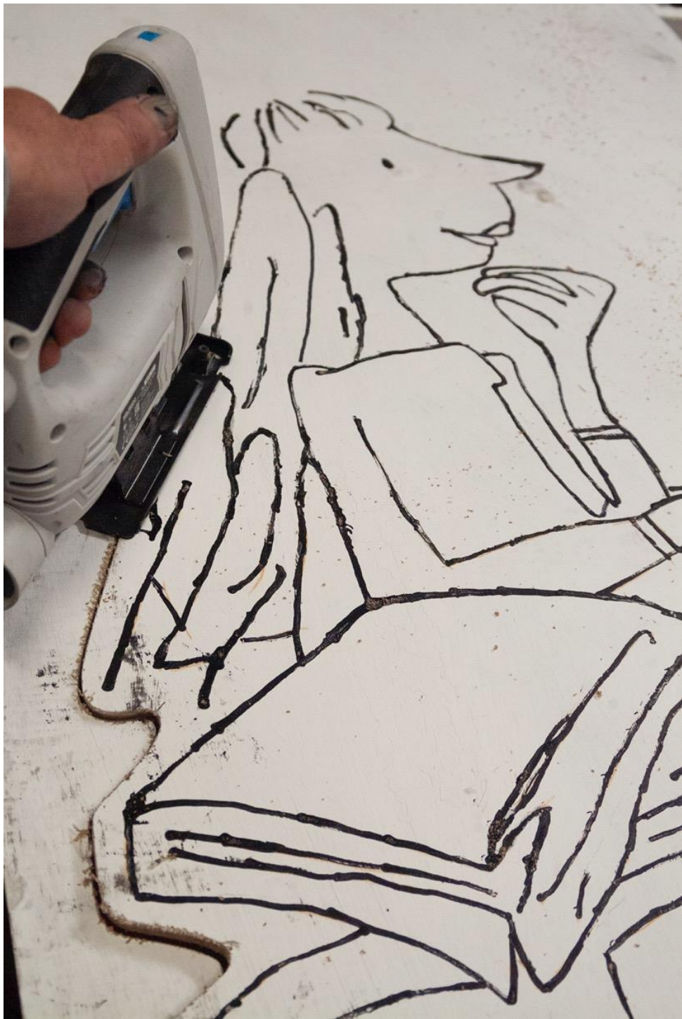
I cut out the drawing using an electric jig-saw, then smoothed the edges with sandpaper.
